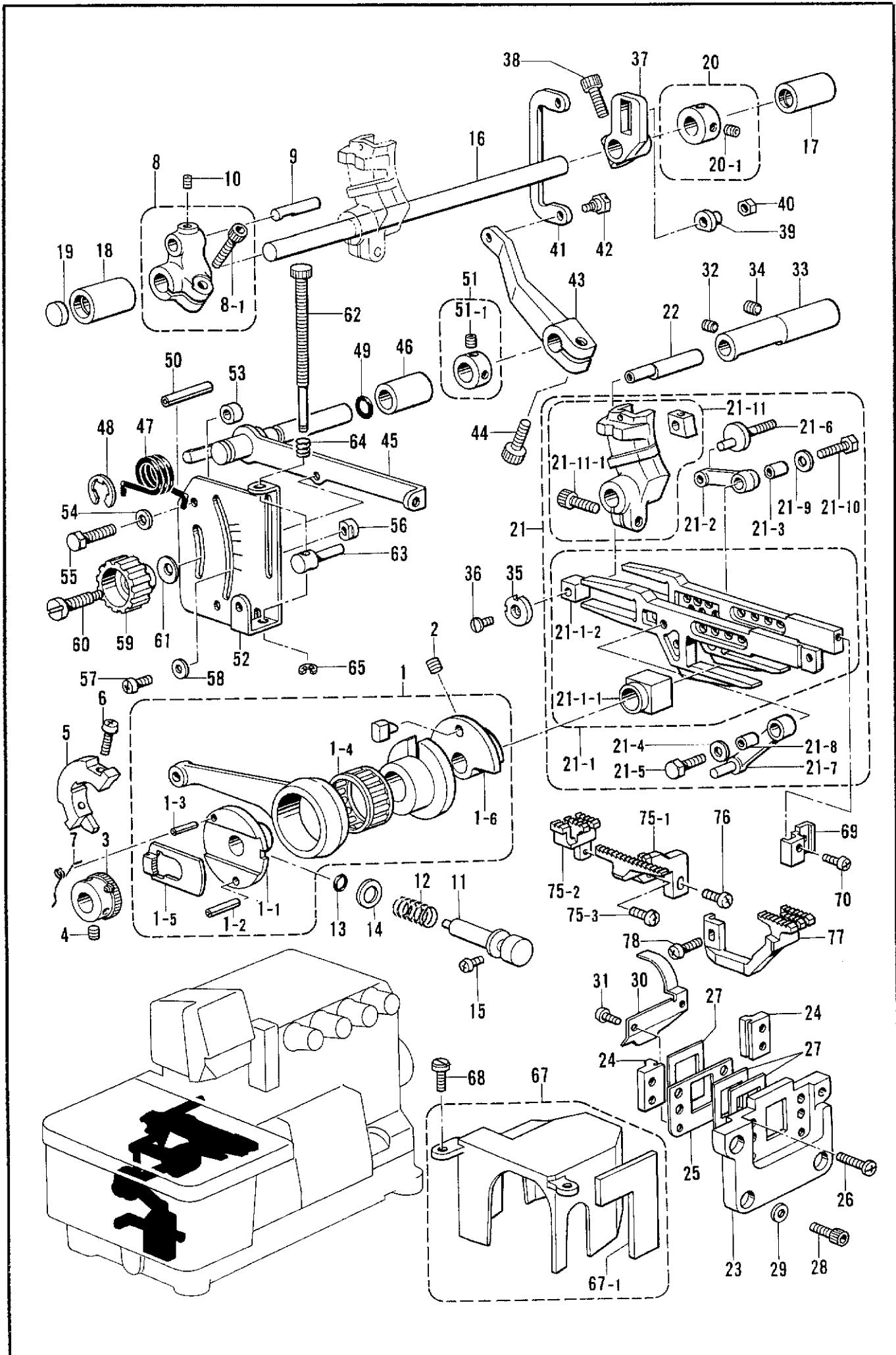
E. 送り関係/Feed mechanism/Transportvorrichtung/
