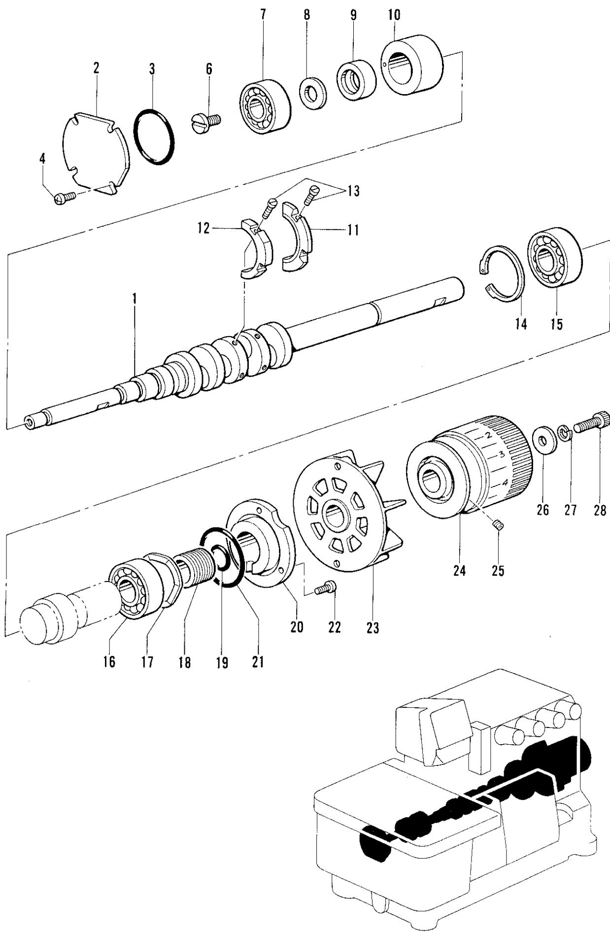
B. 駆動軸関係/Crank shaft mechanism/Kurbelwelle/
