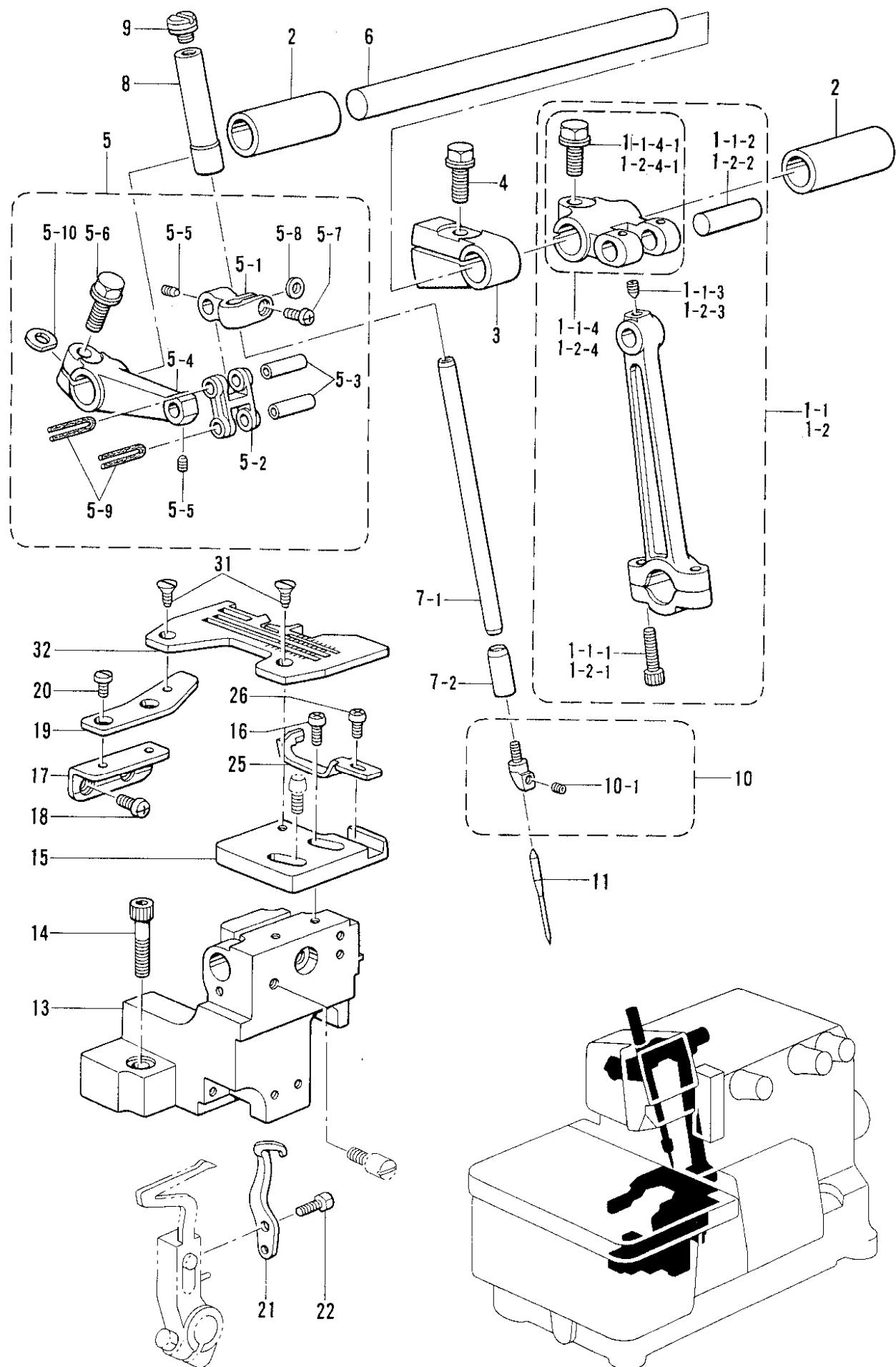
C. 針棒関係 /Needle bar mechanism/Nadelstangenvorrichtung/
