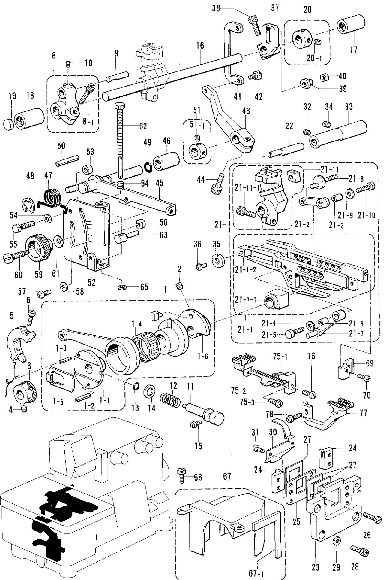
E. 送り関係/Feed mechanism/Transportvorrichtung/
